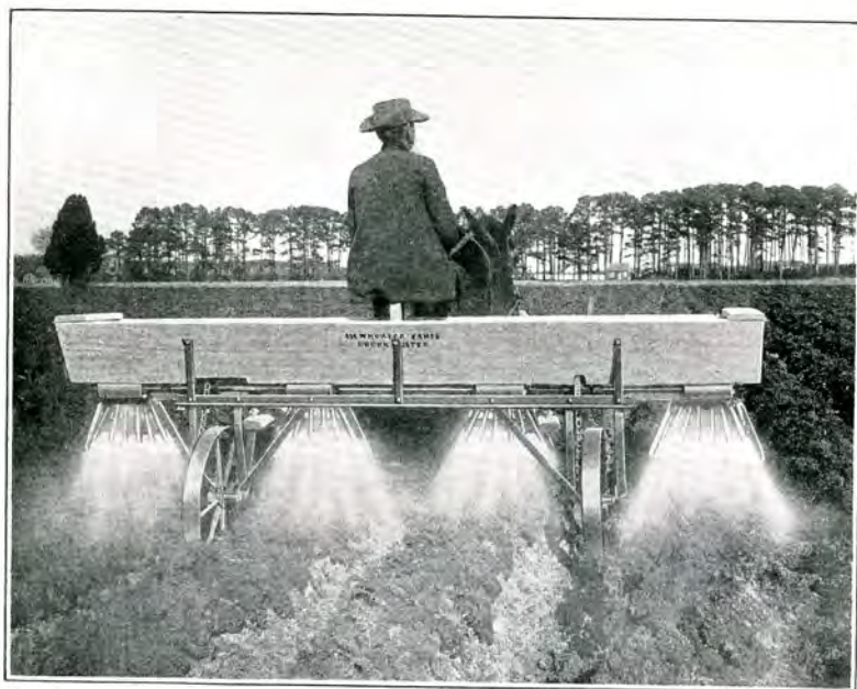
Showing Four-row Duster at Work.
